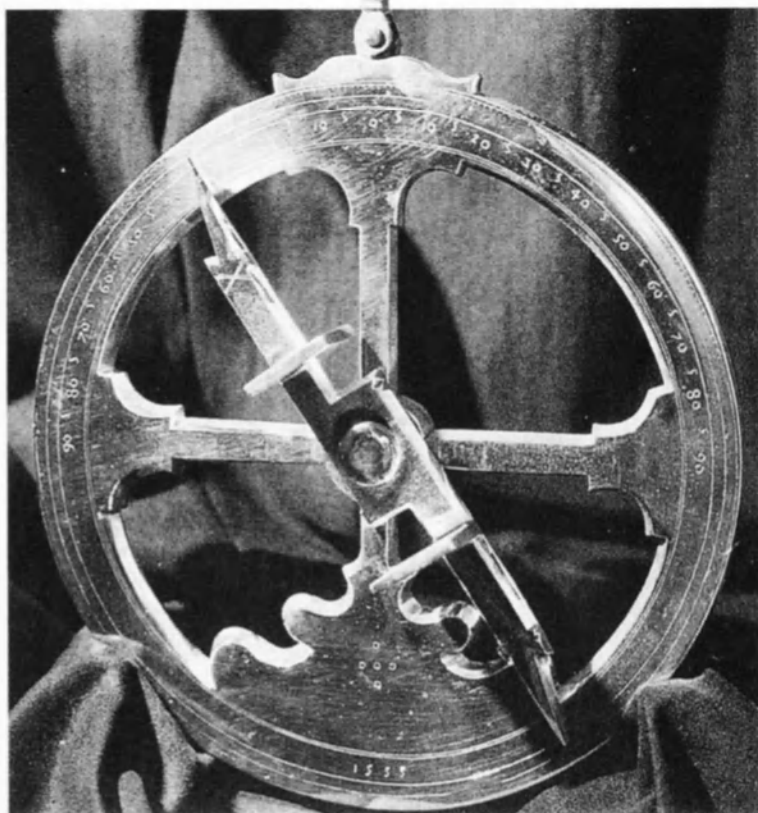
The Portuguese were the first sailors to use the astrolabe, a device for taking the altitudes of celestial bodies, as a navigational instrument. This 16th-century example is preserved in Lisbon's Maritime Museum.
